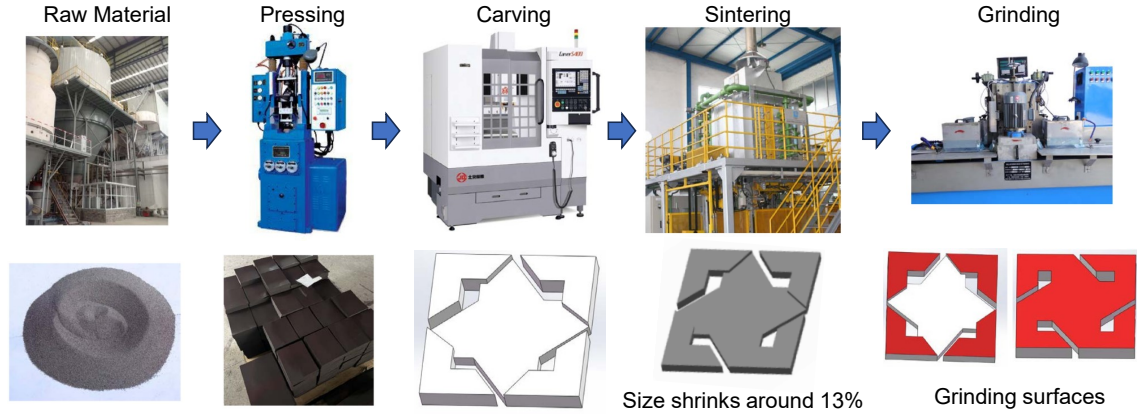
Figure 3.16: Conceptual manufacturing process of magnetic components with customized geometries, provided by ITG Electronics. The carving precision determines how closely the fabricated shape matches the intended design. During sintering, dimensional shrinkage occurs and must be accounted. The effectiveness of grinding directly impacts the flatness and quality of contact surfaces, which are critical for achieving tight assembly and minimizing unintended air gaps.
