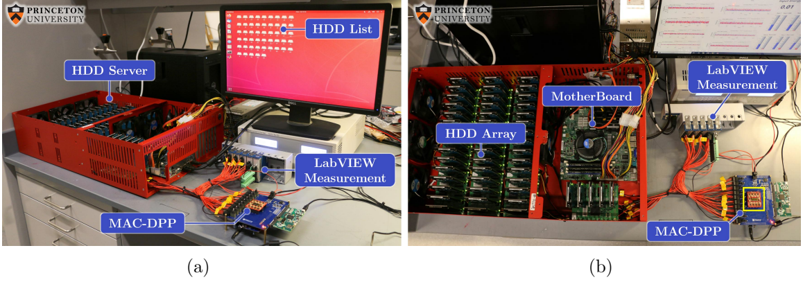
Figure 4.42: (a) Side view and (b) top view of the HDD server testbench supported by the MAC-DPP converter.
